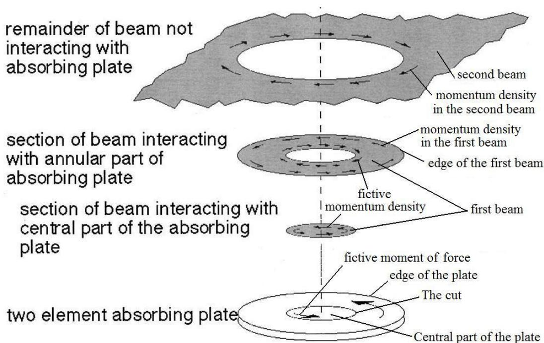
**Fig. 1.** When suspended in a circularly polarized plane wave, a two element absorbing plate comprising a central disc and outer annulus experiences a torque on both components. The torques arise from the effective aperturing of the light beam, such that the large intensity gradient at the perimeter of the plates results in azimuthal components to the momentum density.
