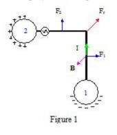
The current creates a magnetic field in space, which exerts a Lorentz force on the wire. The Lorentz force,  $\mathbf{F}_1$  and  $\mathbf{F}_2$ , being perpendicular to the current, is in the x direction on arm 1 and the y direction on arm 2. The two arms are of equal length and the forces on them have the same magnitude *F*. So, the resultant force  $\mathbf{F}_r$  is:
